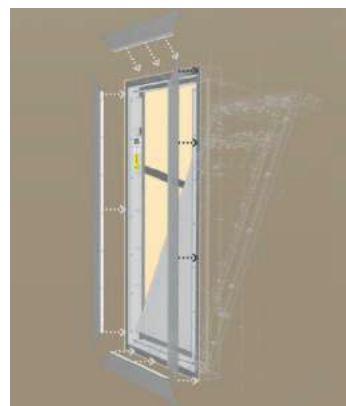
A bead edge profile is fixed to align with the opening edge to allow a plaster finish to be skimmed up to the opening.
